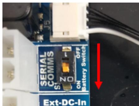
Figure 11. Battery switch ON position
