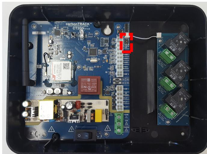
Figure 10. Battery switch location
