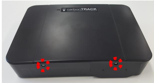
*Figure 1. Remove cover securing screws*
